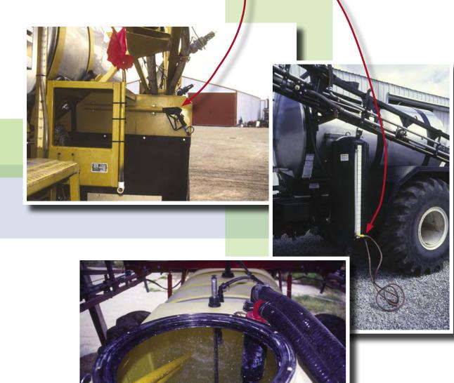
This spray tank has a built-in washer system.
