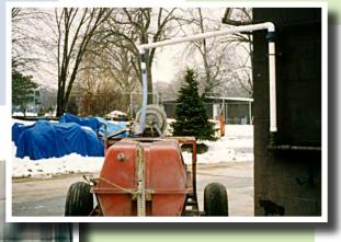
A "swing arm" elevates the hose above the tank in each of these examples.
