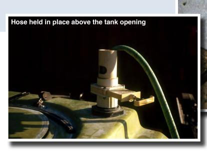
This is an example of a simple, innovative device built to ensure an air gap. It is constructed of three steel prongs (only two visible) and two pieces of iron long enough to fit across the biggest tank opening you have. The prongs fit into the tank and are held in place by the weight of the iron crossbar. Notice the handy quick-connect mechanism between the hose and the air gap device.
