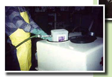
The tank above has been modified with a rinse jet that fits into the opening of a plastic jug; the rinsate drains directly into the spray tank.
