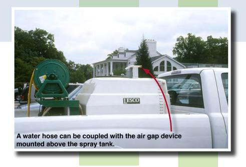
A permanent air gap device is secured to the sprayer lid with four bolts; a quick-connect mechanism facilitates connection of the hose to the device.
