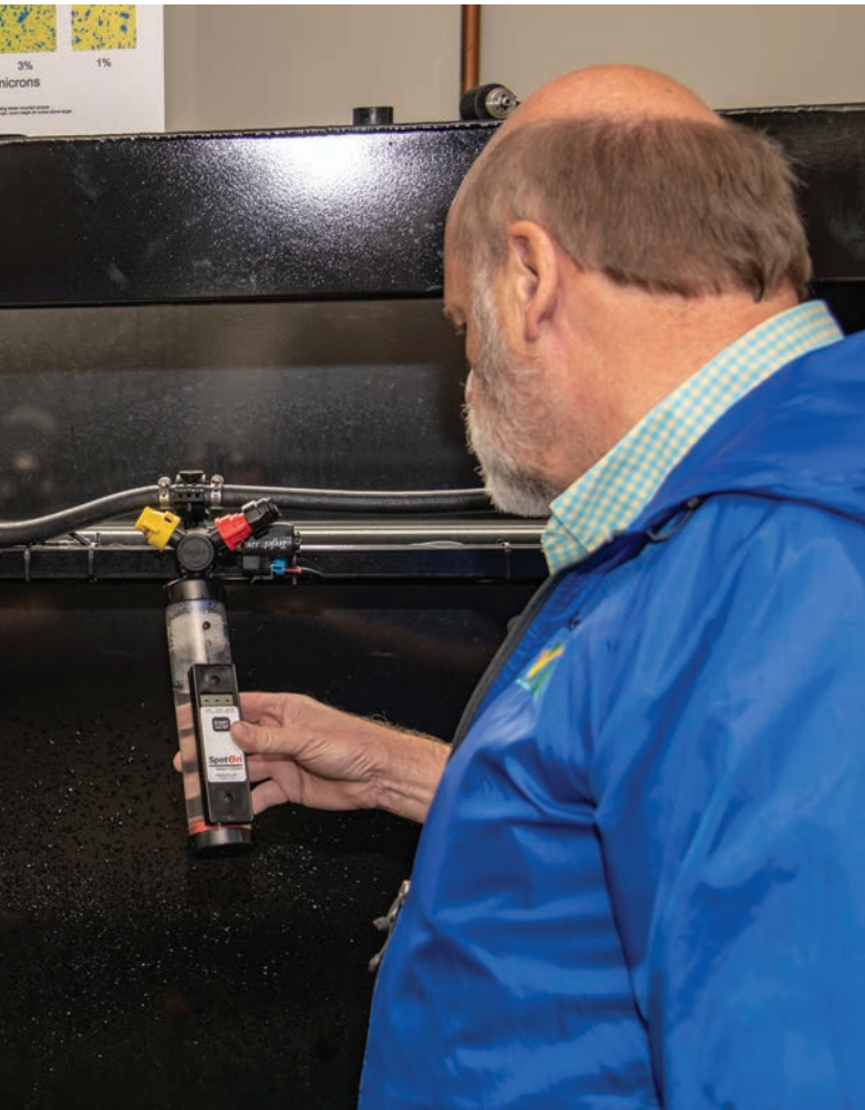
This photo shows the flow rate of water being tested with a SpotOn Sprayer Calibrator. The SpotOn unit on the left displays the flow as ounces per minute (39), while the unit on the right displays gallons per minute (0.31).
