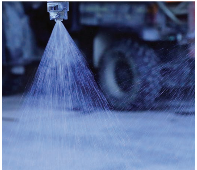
Adjacent nozzles overlap the spray pattern of one tapered flat fan nozzle.
