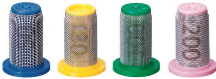
Screens are color-coded to help identify mesh sizes. More recently manufactured screens are also marked their mesh size for quicker identification. This photo shows that a blue 50-mesh screen, a yellow 80-mesh screen, a green 100-mesh screen, and a pink 200-mesh screen.
