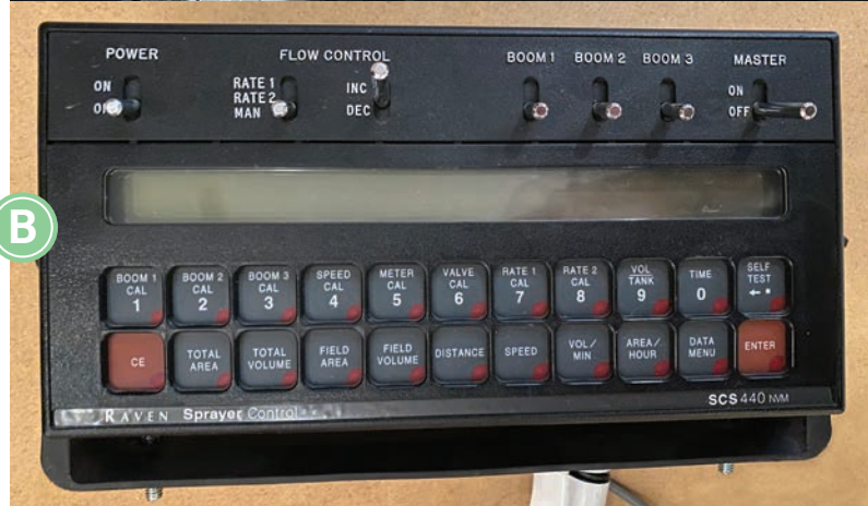
Most sprayers today are equipped with an automated rate controller integrated into the cab's computer system (A), but it was a separate module "box" in the early days of its adaption (B).
