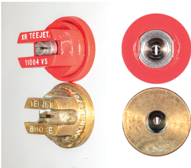
These photos look into the nozzles toward the exit orifices of a conventional tapered flat fan (top, red stainless-steel nozzle) and an even flat fan (bottom, brass nozzle). Notice the differences in the shape of the exit orifices and the width of the cuts of the tapered flat fan (red nozzle) and the even flat fan (brass).
