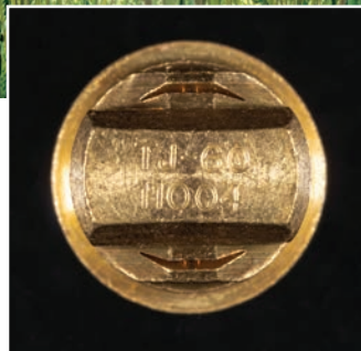
The two exit orifices on this nozzle create a symmetrical flat fan pattern with one spray directed forward and the other backward. The exit orifices are identical in terms of droplet size and flow rate (top and bottom).
