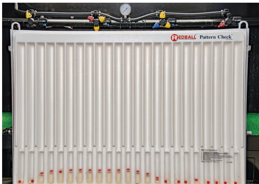
(Below) This photo shows the overlap between nozzle spray patterns that is required to compensate for tapered or reduced volumes along the outer edges of the spray pattern.
