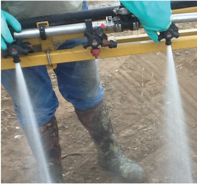
Without a nozzle, the water comes out like a water hydrant, which would serve no purpose in the application process.
