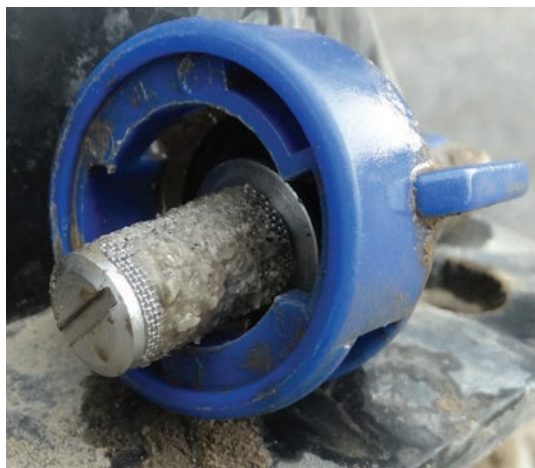
(Left) This stainless-steel screen uses a spring ball-valve to reduce dripping out of the nozzle. This is important if a nozzle body doesn't have a rubber diaphragm valve above the tip as shown in the photo on the right. As a general rule, do not combine a spring ball valve screen with a nozzle body that has a diaphragm valve.
