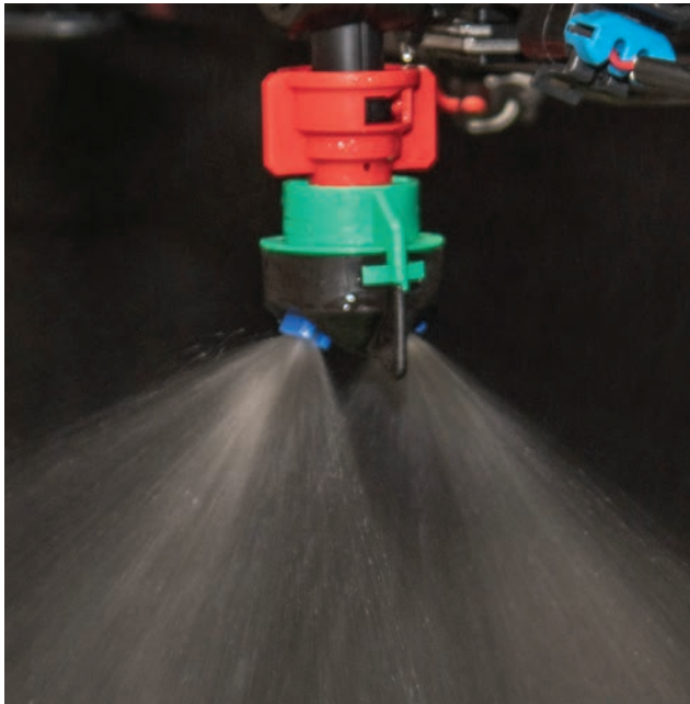
This nozzle body can hold two nozzles oriented forward and backward relative to the sprayer's direction of travel.
