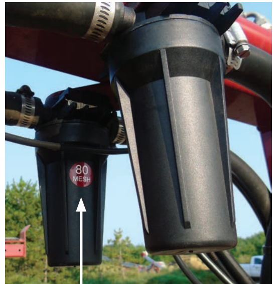
Screens can be used for inline filters for each boom section, in each nozzle body, or both. Applicators with large commercial booms that have numerous nozzle bodies and up to five spray tips on each nozzle body try to avoid using screens in each spray tip cap. This reduces the number of parts they need to clean and inspect.
