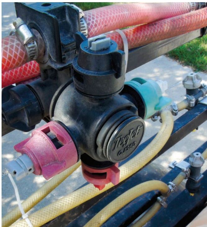
This photo shows different colored caps with different colored nozzles. In this case, the colored caps are randomly used to attach the nozzles to the boom. Color caps offer no visual advantages over standard black caps when used in this manner.
