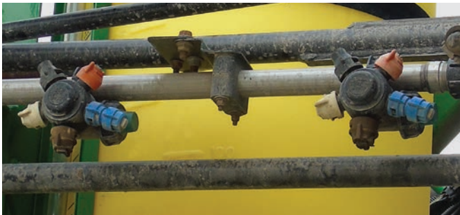
When installing nozzle tips on turrets, make sure to place each tip in the same order on each turret. This will speed the transition to a new nozzle and reduce any chance for error in selecting the wrong nozzles.
