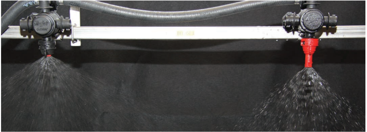
Two different nozzles working under the same pressure can produce remarkably different droplet sizes.
