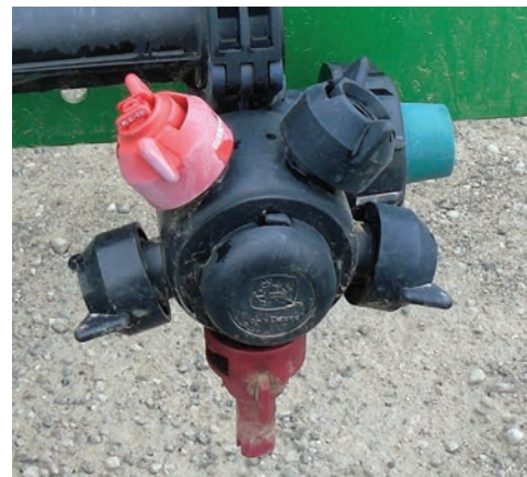
By twisting the turret, applicators can quickly switch nozzles when crops or environmental conditions change.
