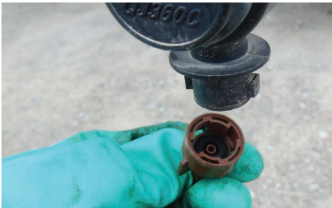
This photo shows a cap with a built-in plastic tip before being placed on the turret.
