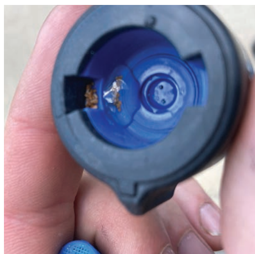
These photos show inline strainers filtering particulate matter in well water. The photo with the nozzle body shows what the nozzle body strainer (screen) filtered out so that the Greenleaf tip would not plug or have the spray pattern compromised by the particulate.
