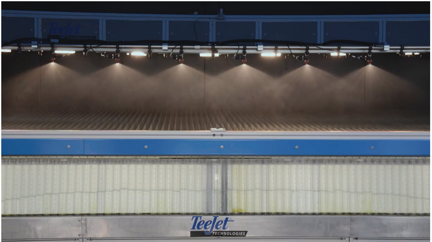
This photo shows an instrument measuring the lateral distribution of a Turbo TeeJet® nozzle with a 110° fan angle and a flow rate of 0.4 gallon per minute. The measured CV is 2.4 percent. Visually, you can tell the nozzles are spaced correctly, because the amount of water collected is almost the same from each nozzle, except for the end nozzles where there was no overlap.
