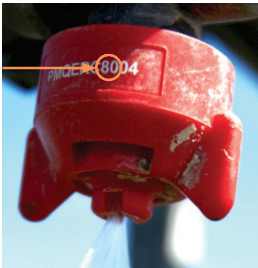
(Top) This nozzle has a 110° angle with a wide fan pattern. (Bottom) This nozzle has a smaller fan angle of 80°.
