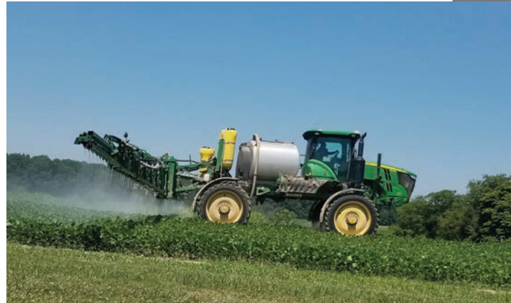
A tapered flat fan does not provide a uniform pattern if the boom is not level across the field. The lowest part of the boom can have gaps and the highest part may allow for spray drift.
