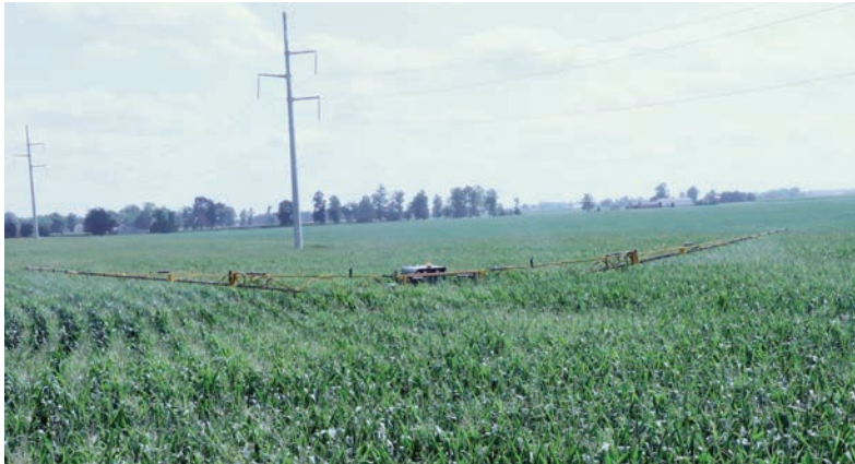
A tapered flat fan does not provide a uniform pattern if the boom is not level across the field. The lowest part of the boom can have gaps and the highest part may allow for spray drift.
