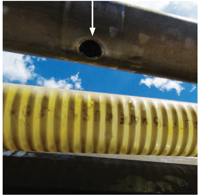
This 90-foot wet boom has 15-inch centers, which means there are 72 evenly spaced holes in which to place the nozzle bodies.
