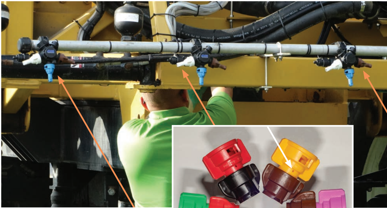
(Top) This boom is equipped with air induction nozzles with nozzle bodies equipped with different flow rates (blue, white, brown).
