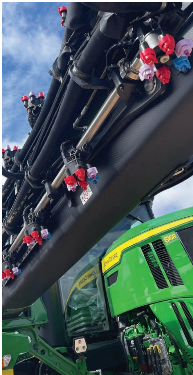
Nozzles are color-coded to reflect industry standards for flow rates (see page 42).
