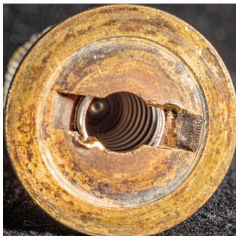
(Left) This stainless-steel screen uses a spring ball-valve to reduce dripping out of the nozzle. This is important if a nozzle body doesn't have a rubber diaphragm valve above the tip as shown in the photo on the right. As a general rule, do not combine a spring ball valve screen with a nozzle body that has a diaphragm valve.
