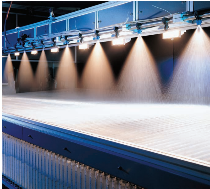
The front view (top) and side view (left) of two patternators show nozzles spraying into plastic compartments where their output will be measured. Lateral distribution is an important measurement to determine the proper overlap required between nozzles.
