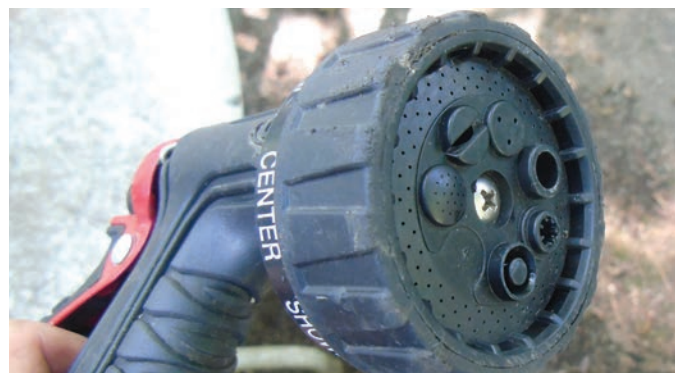
A turret garden hose sprayer has different spray patterns. Selecting the appropriate orifice allows you to perform various functions, including watering plants from a distance, gently misting shallow-planted seeds, or cleaning surfaces with a concentrated stream.
