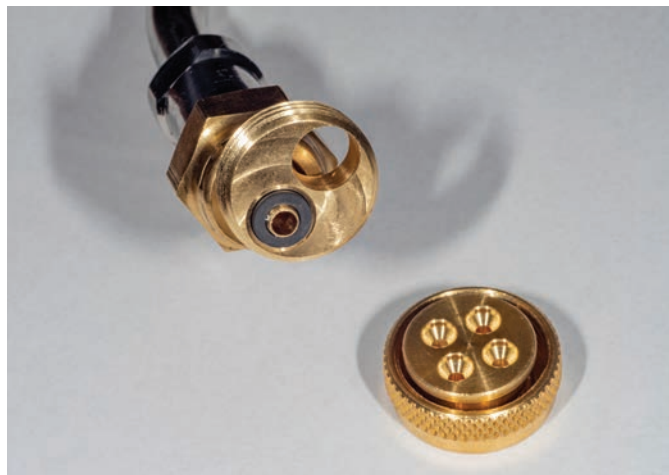
A brass nozzle like this one is commonly used by the pest control industry with manual pump-up sprayers. The nozzle shown here can be set to four positions depending on the desired spray pattern.
