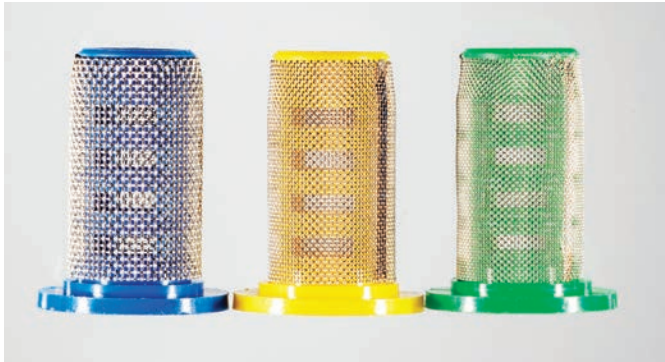
A screen's width determines what size materials will pass through it. The blue 50-mesh screen has larger openings than the yellow 80-mesh screen, which has larger openings than the green 100-mesh screen.
