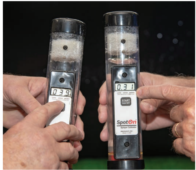
This photo shows the flow rate of water being tested with a SpotOn Sprayer Calibrator. The SpotOn unit on the left displays the flow as ounces per minute (39), while the unit on the right displays gallons per minute (0.31).
