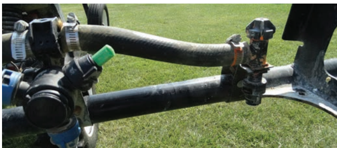
Different cap designs hold and lock specific nozzles in place.
