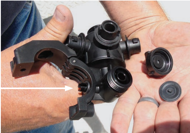
The stem on this new turret (arrow) fits into the hole in a wet boom, which is then clamped in place.
