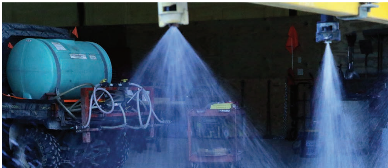
(Below) A 110° nozzle in use. Both a 110° and 80° spray nozzle are predicated on the width of the exit orifice. (Right) Most nozzles list their spray width angles as part of their descriptions.
