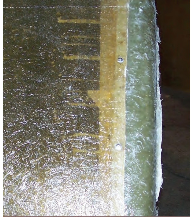
(Top) Individual rivets in a fiberglass tank. These tanks (12 feet diameter x 10 feet tall) are ready for the final fiberglass layers to be added (bottom). The three main parts of the tank — bottom, sidewall, and top — are clearly visible.
