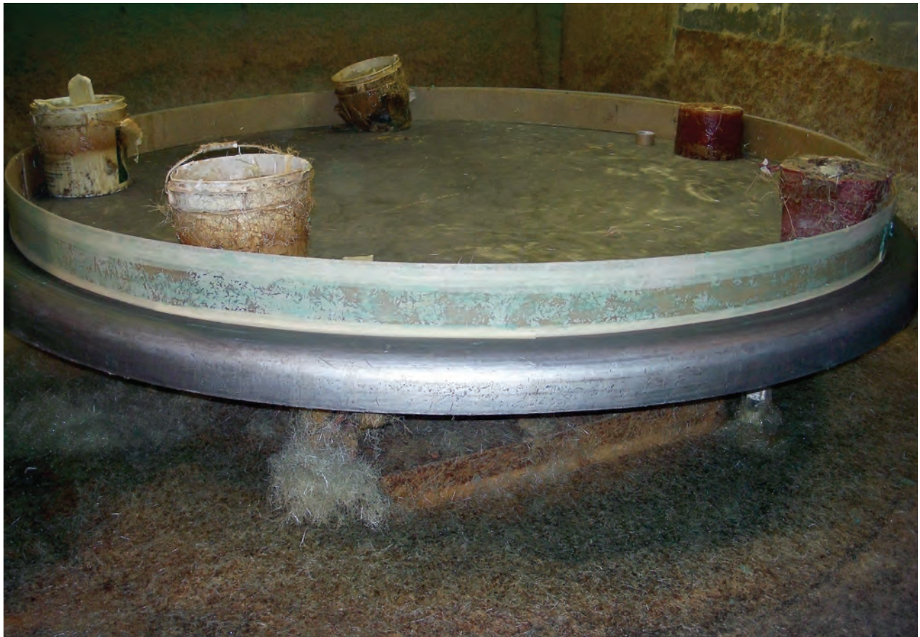
A manufacturer prepares the mold for the top of a fiberglass tank.
