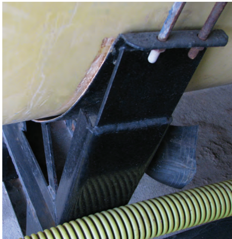
(Bottom left) A soft insert separates this tank from metal. (Bottom right) The soft insert for this tank fell out and the tank was damaged when it rubbed against the metal frame.
