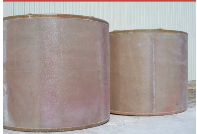
(Top) Individual rivets in a fiberglass tank. These tanks (12 feet diameter x 10 feet tall) are ready for the final fiberglass layers to be added (bottom). The three main parts of the tank — bottom, sidewall, and top — are clearly visible.
