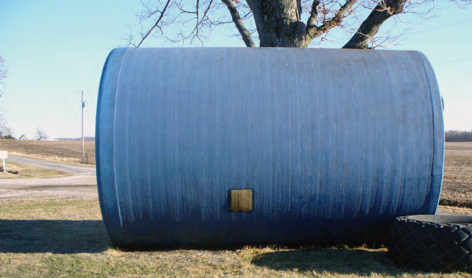
A simple fiberglass repair. Painting over the fiberglass patch would have helped protect it against ultraviolet light.
