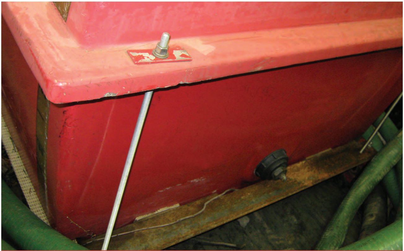
These metal rods link the fiberglass tank to the metal frame.
