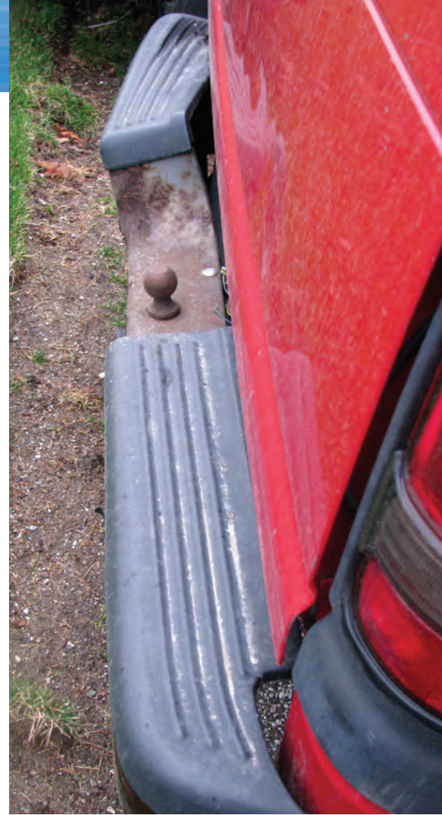
These bumpers have been twisted from towing excess weight.
