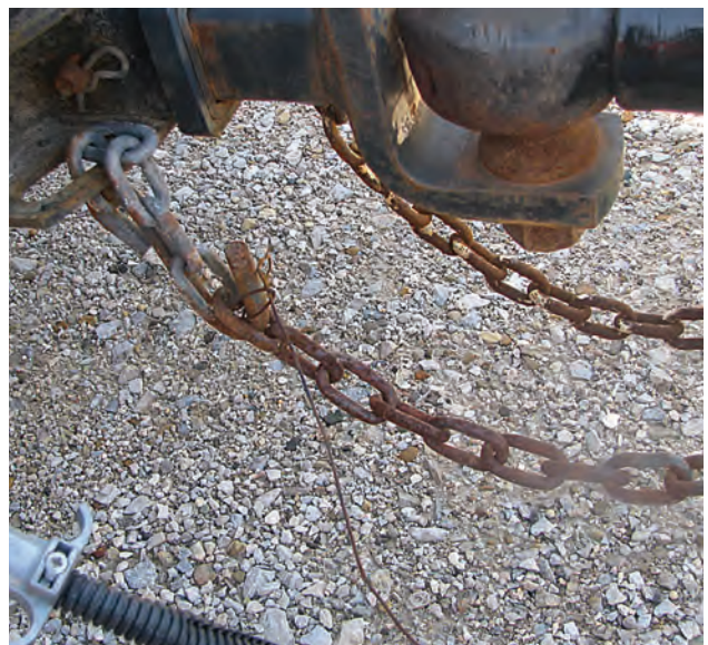
The wire is so rusted that it would pull apart before it could activate the emergency brake.
