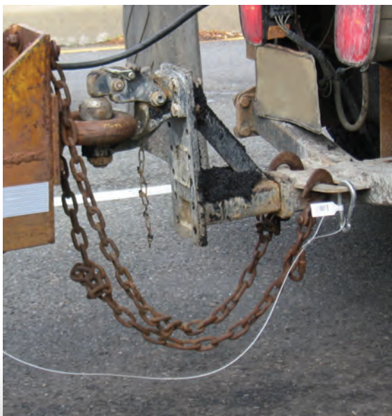
Always connect the emergency brake cable directly to the towing vehicle.
