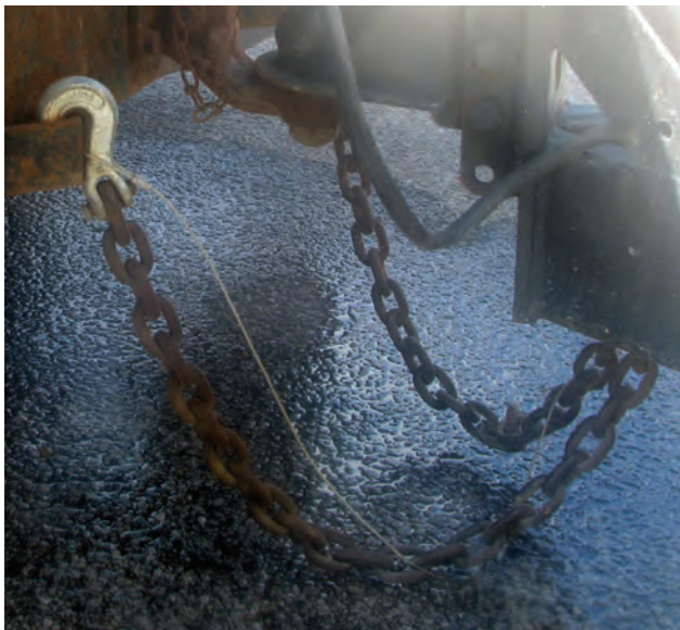
This emergency trailer brake cable is improperly hooked to the chain.
