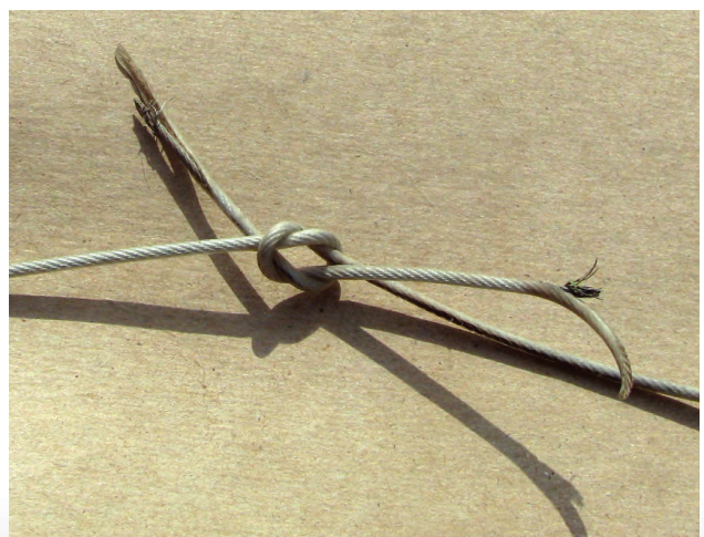
Do not tie two parts of a broken cable together. If a cable breaks, replace it.
