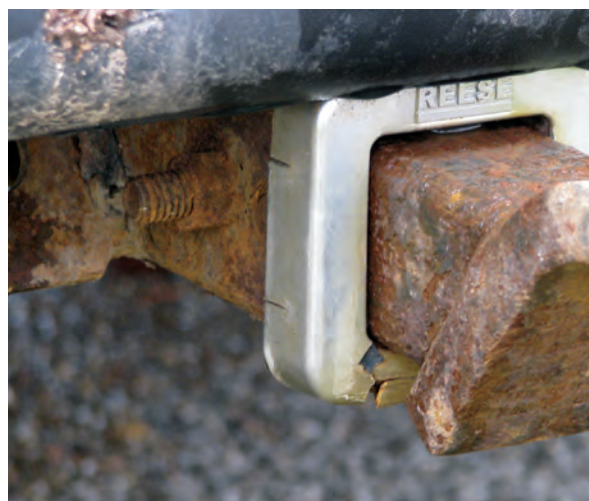
A hitch pin that has rusted in place (bottom), and one designed to be locked (top).
