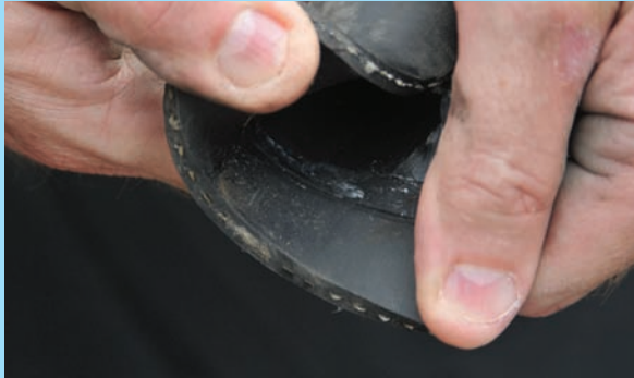
Clamp marks (right) and fitting marks (below) on hoses.
