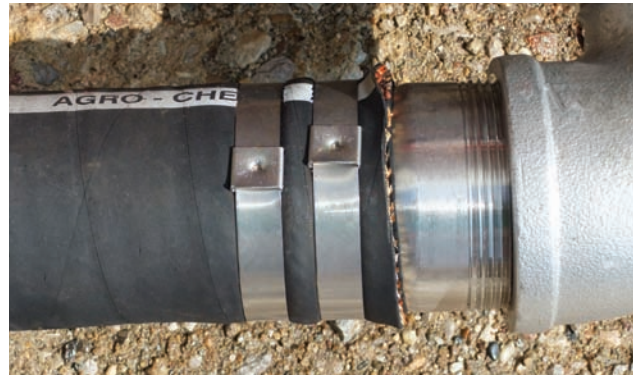
An advantage of band-it hose clamps is that they will not catch on other objects when the hose is mobile.
