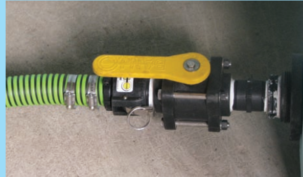
Two clamps (below) provide additional protection inexpensively. Throughout the season, make sure worm gear and T-bolt clamps are properly tightened.
