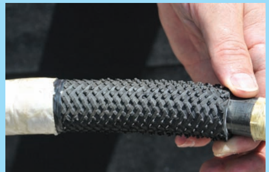
3. First layer of reinforcing fibers.
