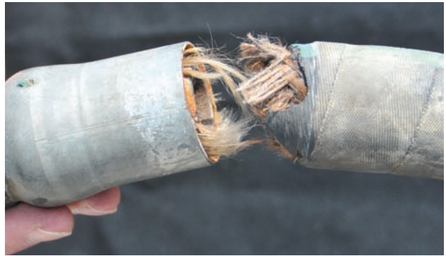
This hose failed where it kinked behind the fitting.
