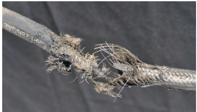
This hose failed where it was subject to continuous abrasion.
