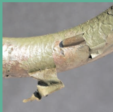
When oil or grease remain on a hose, it can create soft spots that weaken a hose's integrity.
