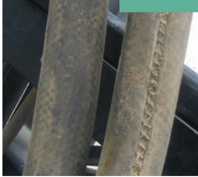
These photos show hoses worn from rubbing. Even covers might not protect underlying hose layers as shown in the photo of the orange hose.
