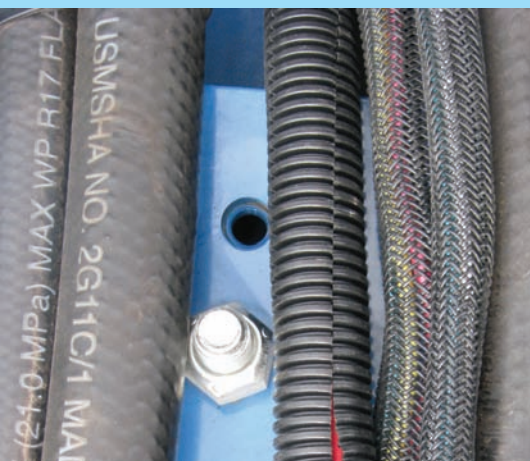
(Above) The hose on the left is not protected and rubbing against a metal bolt, which can cause it to break down prematurely.
