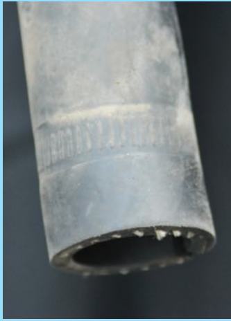
Clamp marks (right) and fitting marks (below) on hoses.
