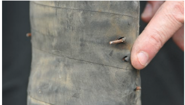
Kinking can permanently pinch the wire braid in hoses.
