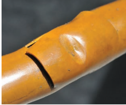
These photos show hoses worn from rubbing. Even covers might not protect underlying hose layers as shown in the photo of the orange hose.
