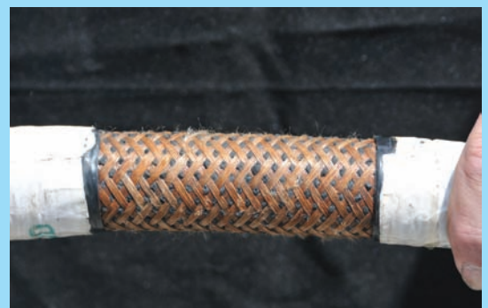
4. Second layer of reinforcing fibers.
