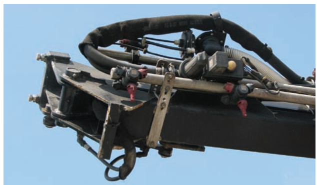
Improperly installed hoses can kink and fail.
