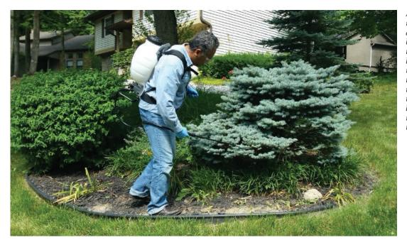
A typical backpack is not very effective for adult mosquito control, because the drops are too large to coat the leaves. A backpack might be useful to treat the boundary between two properties because the larger droplets pose less risk for off-target movement of the insecticide. I.
