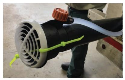
An example of securing a nozzle onto a backpack mist blower.
