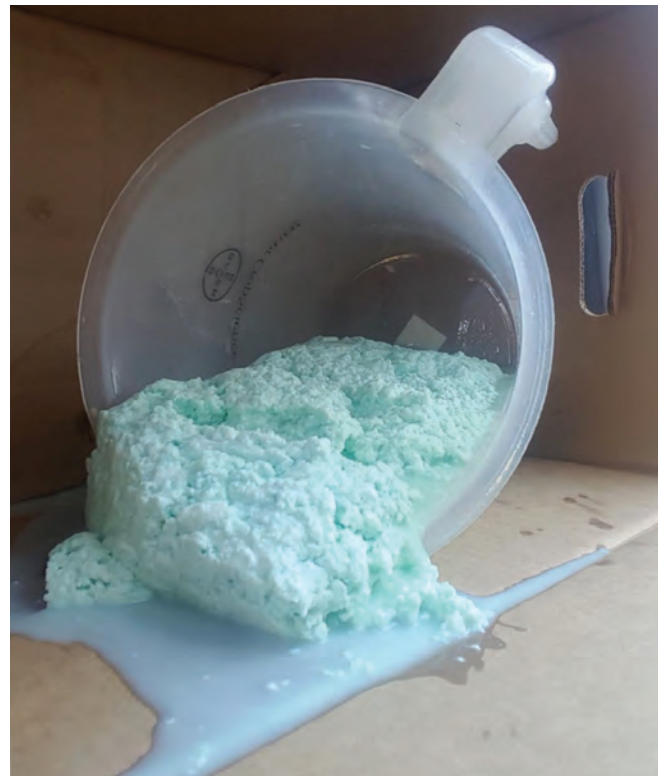
This product did not go back into solution once mixed. It is a candidate for disposal.
