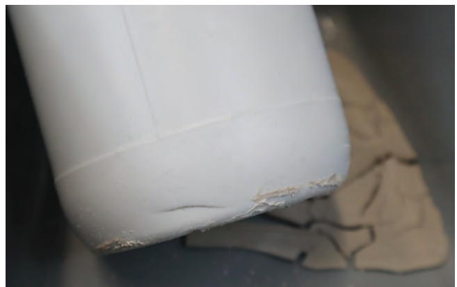
Manufacturers test all parts of their product's packaging to make sure the materials are compatible with the formulation. (Top) Testing the cap foil. (Middle) The yellow on the bag is a discoloration of the plastic because of product permeation. (Bottom) A plastic container that has failed.
