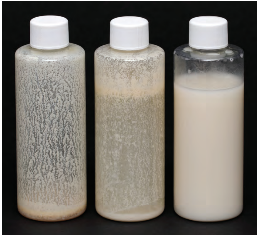
Temperature extremes may cause active or inert ingredients to precipitate out, causing poor product performance.
