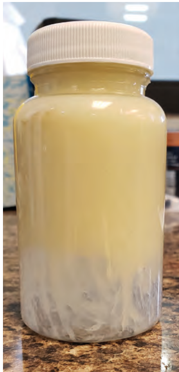
The jar test on this old product shows that it is a candidate for disposal.
