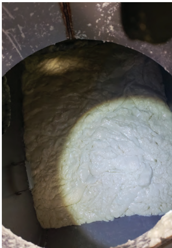
An unstable formulation concentrate can cause major problems in a spray tank.
