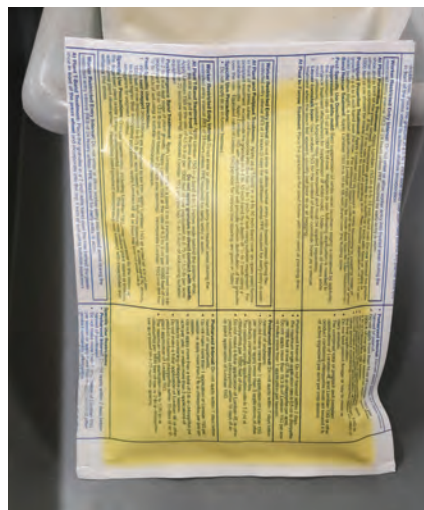
Manufacturers test all parts of their product's packaging to make sure the materials are compatible with the formulation. (Top) Testing the cap foil. (Middle) The yellow on the bag is a discoloration of the plastic because of product permeation. (Bottom) A plastic container that has failed.
