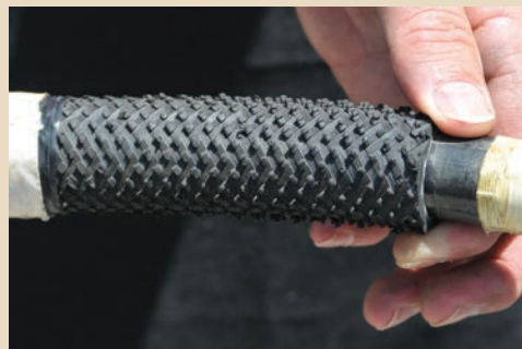
3. First layer of reinforcing fibers.
