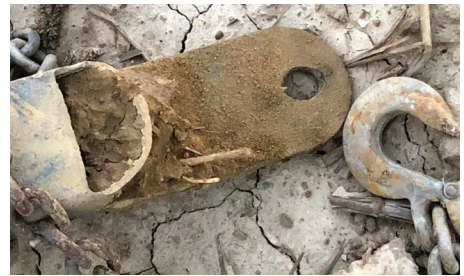
These photos show an ammonia release that resulted from a failed hitch. The pin came out and the hose was pulled apart. The soil around the tank was frozen, but was able to be excavated and then incorporated back into the same field.
