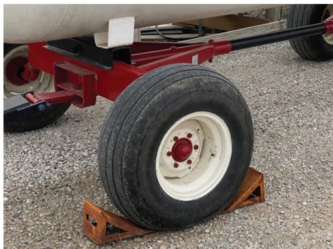
These chocks prevent the forward and backward movement of the nurse tank.
