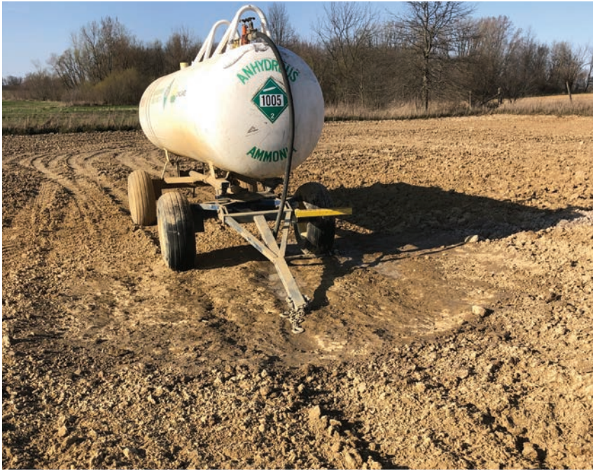
These photos show an ammonia release that resulted from a failed hitch. The pin came out and the hose was pulled apart. The soil around the tank was frozen, but was able to be excavated and then incorporated back into the same field.
