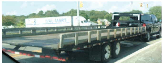
The side rails on this trailer were installed after purchase. Adding a sign or making any modifications to the trailer makes it unique. Be sure to document these changes.
