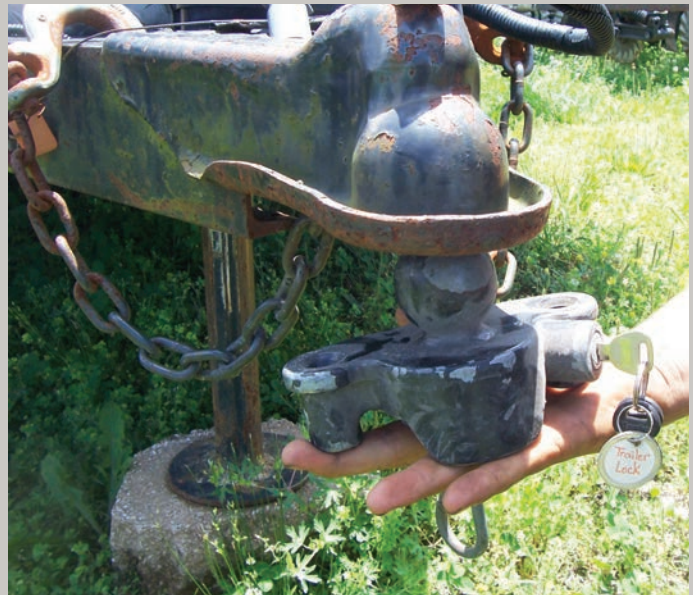
The coupler insert on a ball hitch lock has a locking mechanism.
