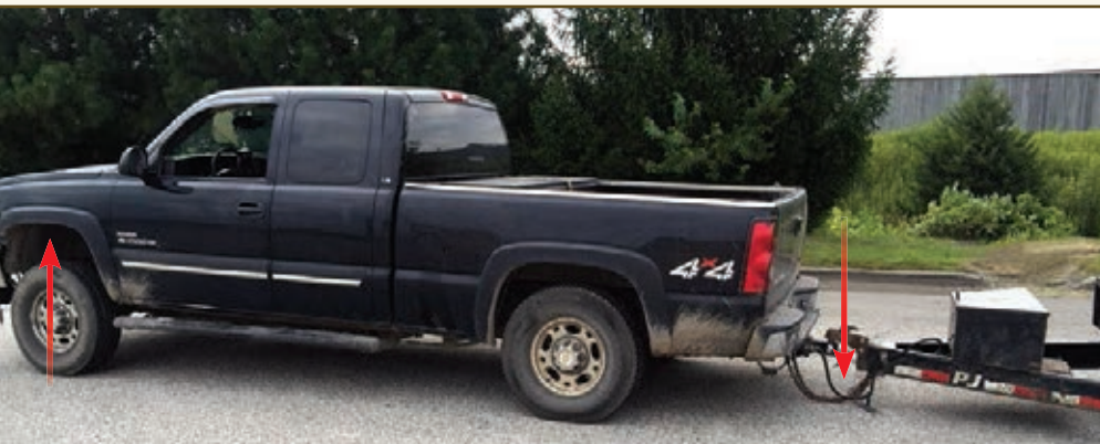
Note how the heavy tongue weight of the trailer forces up the front of the towing vehicle.
