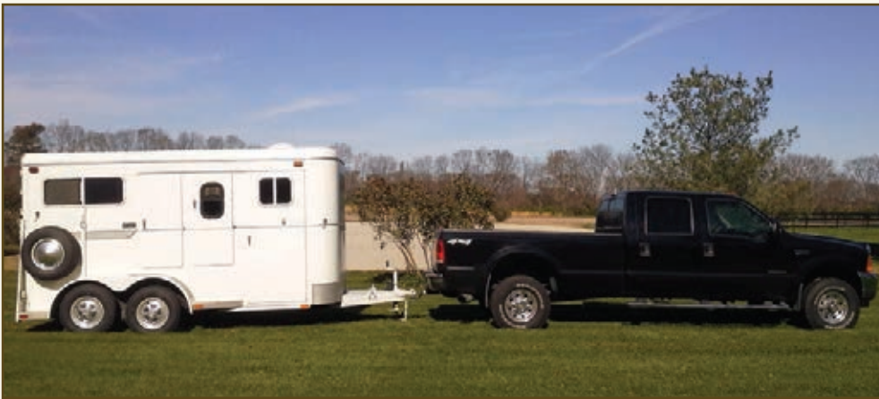
A horse trailer with a tagalong (weight-carrying) rig couples to a ball mounted at the rear of the truck.
