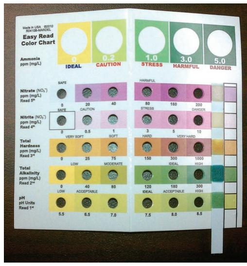
A water sampling kit uses litmus paper, which changes color to measure water pH and hardness.
