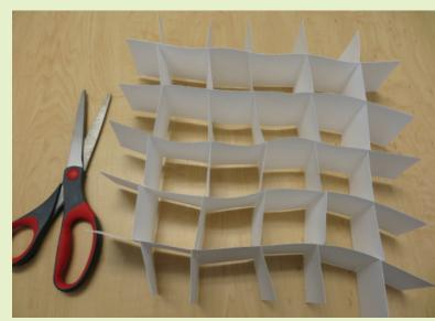
After making several strips with slits, fit the strips together using the slits to make baffles.
