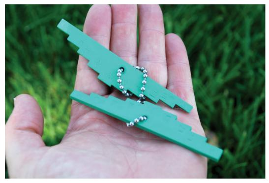
A third hole-type spreader should come with a calibration gauge. This gauge has stepped increments of 1/32 inch to allow the applicator to accurately measure the size of the opening. Use the gauge (not the numbers on the operating lever) to accurately document the opening size. After you obtain the desired spread pattern, document the step number and the product information for future reference.
