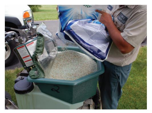
When calibrating the spreader pattern, make sure to use the same fertilizer or pesticide you plan to apply.
