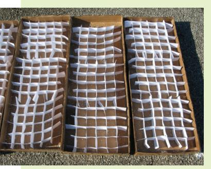
These custom 1-foot by 3-feet collection boxes were made from cardboard scraps and packing tape.
