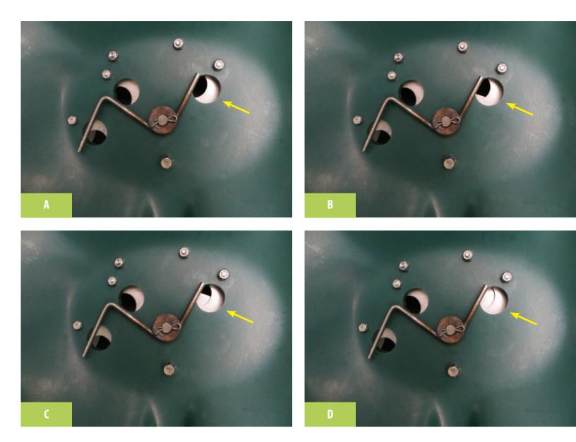
Some spreaders use the third hole to adjust the spreader pattern (A). Whether the third hole is open (A), closed (D), or somewhere in between (B-C) affects how the product is distributed onto the moving impeller.
