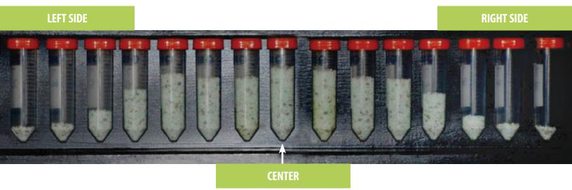
This is a good spreader distribution pattern. Although not perfect, this might be as close as you can get to an ideal pattern. Make sure that the fertilizer distribution is evenly balanced on the left and right sides of the center. The arrow marks the center collection tube and direction of travel.
