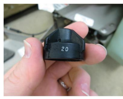
You can adjust the pressure from 20 to 30 psi on the diaphragm-type antidrip valve on Permagreen® models. This slightly increases the effective spray width.
