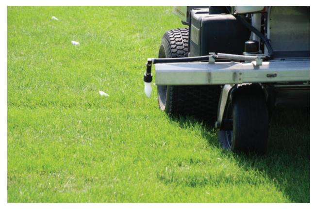
This boom sprayer has a foam marking system that marks the edges of the spray pattern.
