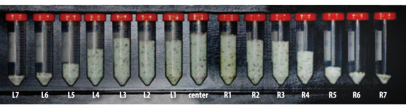
The effective spread width for this spreader is the distance from the box that corresponds to the L4 tube to the box that corresponds to the R4 tube.
