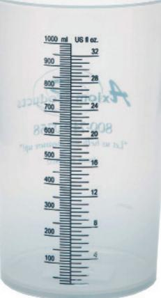
Quart and pint measuring containers that have printed markings for each whole and half fluid ounce are ideal for calibration measurements.
