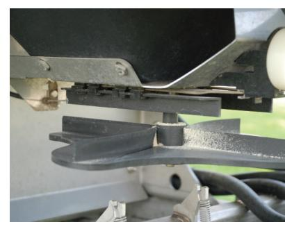
A rotary spreader's distribution pattern can change when granular dust builds up on the spinner (impeller). Clean the spinner on a regular basis to keep the application accurate.
