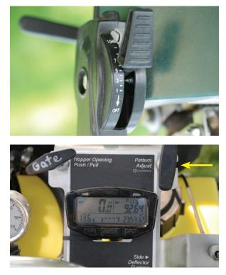
The pattern adjustment lever varies by spreader model. You control the pattern on a PermaGreen® with the third hole adjustment operating lever (top). You control the Z-Spray Intermediate® (bottom) with a pull knob.
