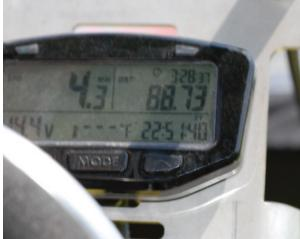
If your sprayer has a speedometer, record the speed that was used during the calibration.
