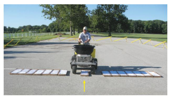
In this example, the spreader is being calibrated for a product with a small granule , so there is no space between the boxes. Closer box spacing with small granules helps you determine the effective spread width more accurately.
