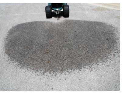
Check the nozzle distribution pattern while the sprayer is parked and spraying at the same RPM and pressure as during the calibration run. This nozzle has a uniform spray pattern.
