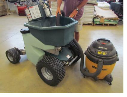
A shop vacuum will help you remove the fertilizer that was left in the hopper. Subtract what's left from the amount you started with to calculate how much fertilizer you applied to the calibration course.
