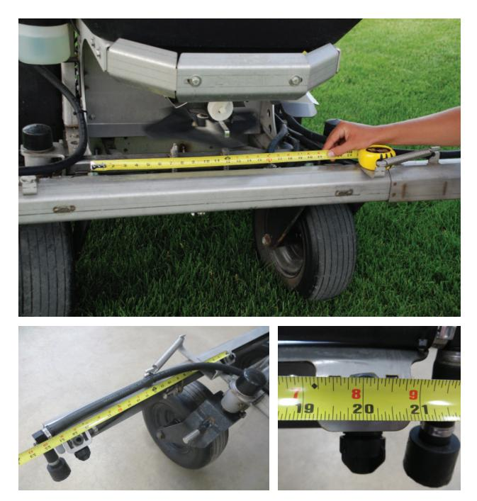
The distance between nozzles may differ between manufacturers, but for each unit the distance between nozzles should be equally spaced.
