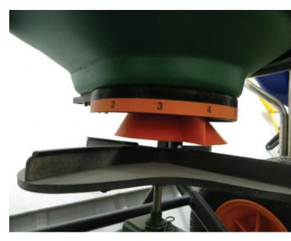
This spreader uses a rotating conical distribution device to adjust where the fertilizer hits the impeller, which adjusts the spread pattern.
