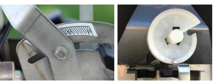
The spreader gate opening lever varies by spreader model. The settings on a PermaGreen<sup>®</sup> (left) are numbered 0 to 30, and the settings on the Z-Spray Intermediate<sup>®</sup> (right) are numbered 1 to 9.
