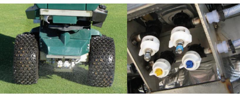
This single-nozzle boomless ride-on sprayer has four nozzles, but it only uses one at a time.
