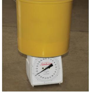
Use a scale like this one or a bathroom scale to weigh the product left in the hopper after the calibration run.
