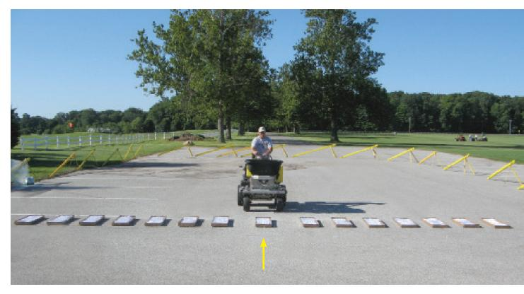
The center box is marked with an arrow. Notice the extra space on either side of the center box to allow room for the wheels. In this example, the spreader is being calibrated for a product with a large granule, so the boxes are placed about 12 inches apart to catch the granules along the entire width of the spread.
