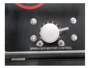
Some units may have a hydraulic impeller motor that can adjust the spread width. When you calibrate one of these units, note the setting you are using. If you adjust this setting you will need to recalibrate.
