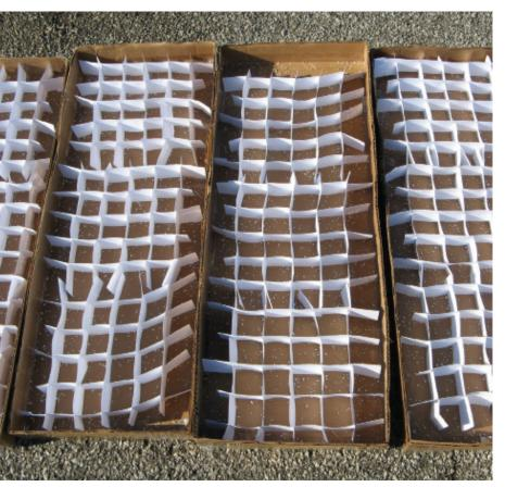
To check a spreader's distribution pattern, place shallow boxes with baffles side-by-side in a line perpendicular to the direction the spreader will travel.
