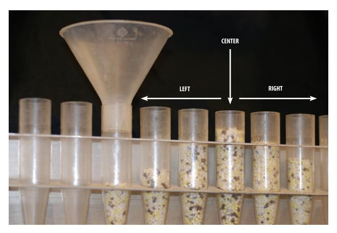
After your calibration run, pour the contents of each box into its own small container. Keep the boxes (and tubes) in order from left to right.
