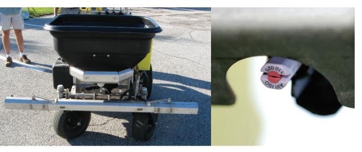
A boom-type ride-on sprayer (left) and one of the nozzles along its boom (right).
