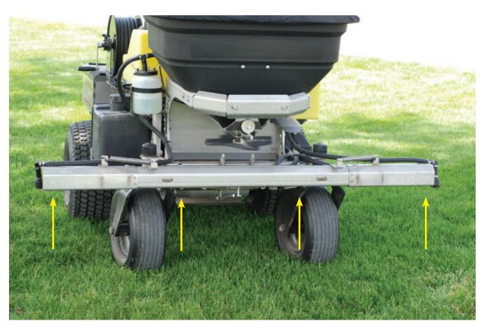
A boom-type ride-on sprayer/spreader with four nozzles. Arrows point to nozzle placement.
