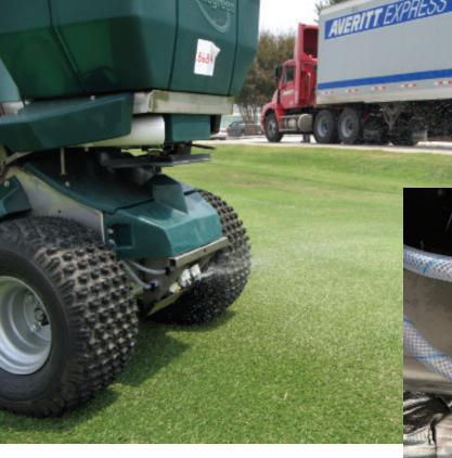
Most single-nozzle (boomless) sprayers actually have a cluster of nozzles under the front center of the sprayer. Although there are multiple nozzles, you should only use one at any time. The ability to select nozzles permits quick and accurate changes in spray width for trim and broadcasting or when changing ground speed. You must calibrate each nozzle and speed combination on the sprayer.
