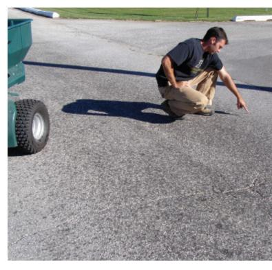
Locate each edge of the spray pattern where the pavement is consistently wet. Measure from edge to edge to get the effective spray width.
