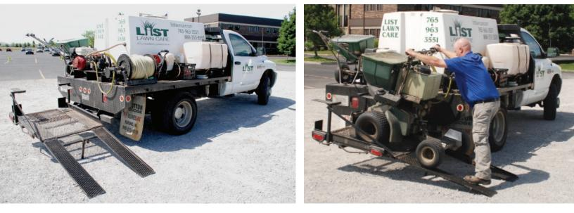
This carrier was specially built to haul ride-on sprayers. Some carriers feature passive restraint systems that improve safety and ease of unloading and loading. These carriers don't require trailers, which means operators can haul ride-on equipment with compact vehicles that are easier to maneuver in residential neighborhoods. Typically, a vehicle needs a heavy-duty hitch to carry these units.
