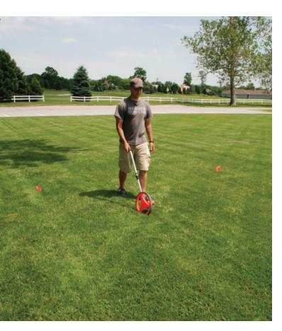
Use a measuring tape or wheel to measure the length of a calibration course.
