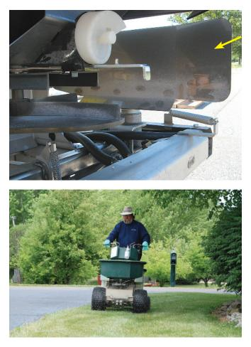
The edge guard (deflector) is a physical barrier that prevents the fertilizer from going onto impervious surfaces. Without a guard, the spreader shown below would apply fertilizer onto the paved surface. Always blow or sweep fertilizer off any sidewalks back into the turf.
